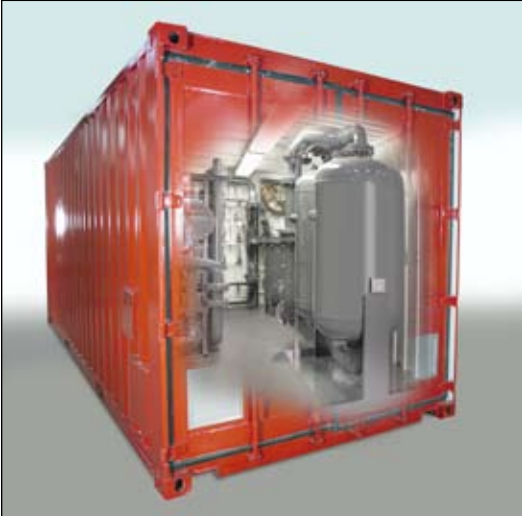
Model FB-12ST15020 rated at 1500 scfm of 95% N2
